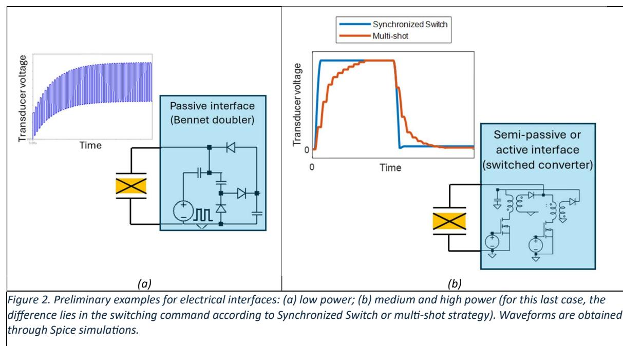
Figure 2. Preliminary examples for electrical interfaces: (a) low power; (b) medium and high power (for this last case, the difference lies in the switching command according to Synchronized Switch or multi-shot strategy). Waveforms are obtained through Spice simulations.
